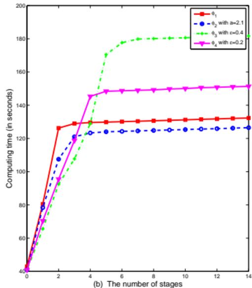
Figure: The performance of multi-stage convex relaxation with  $p = 3980$
